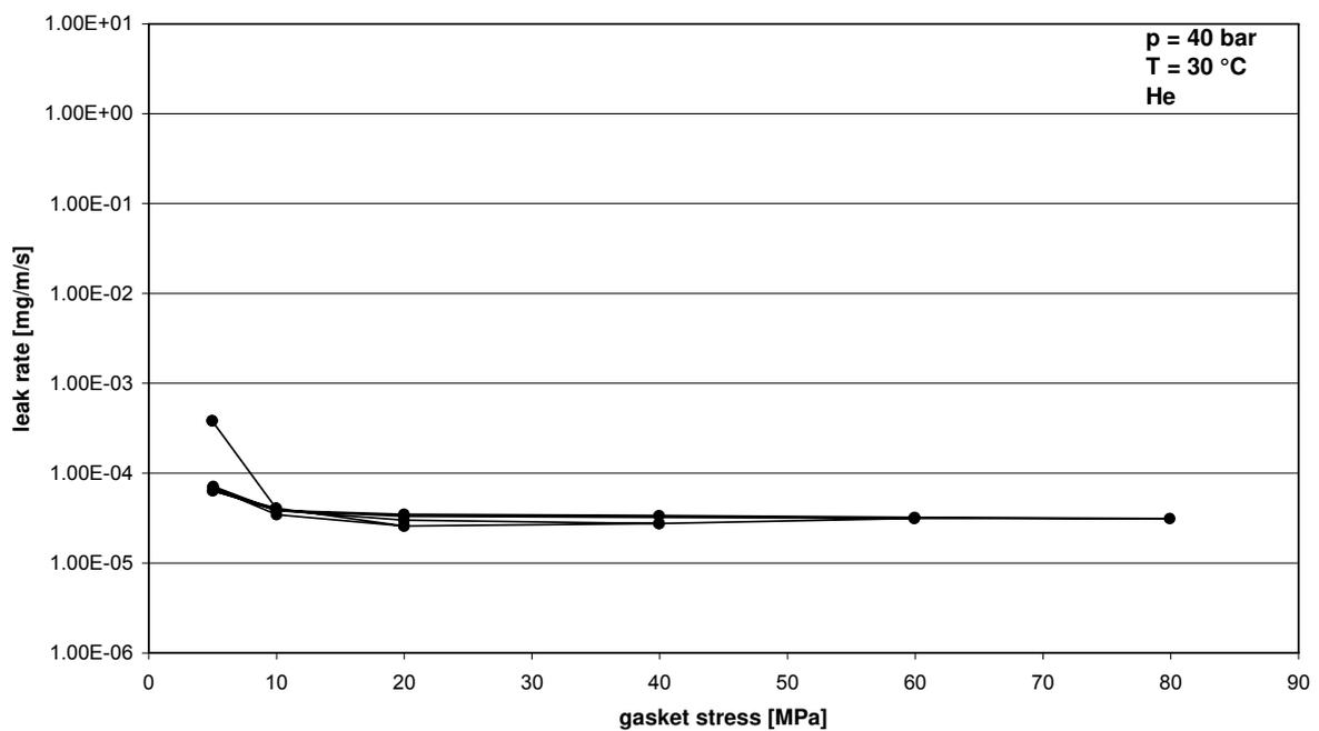
Leakage test according EN 13555
