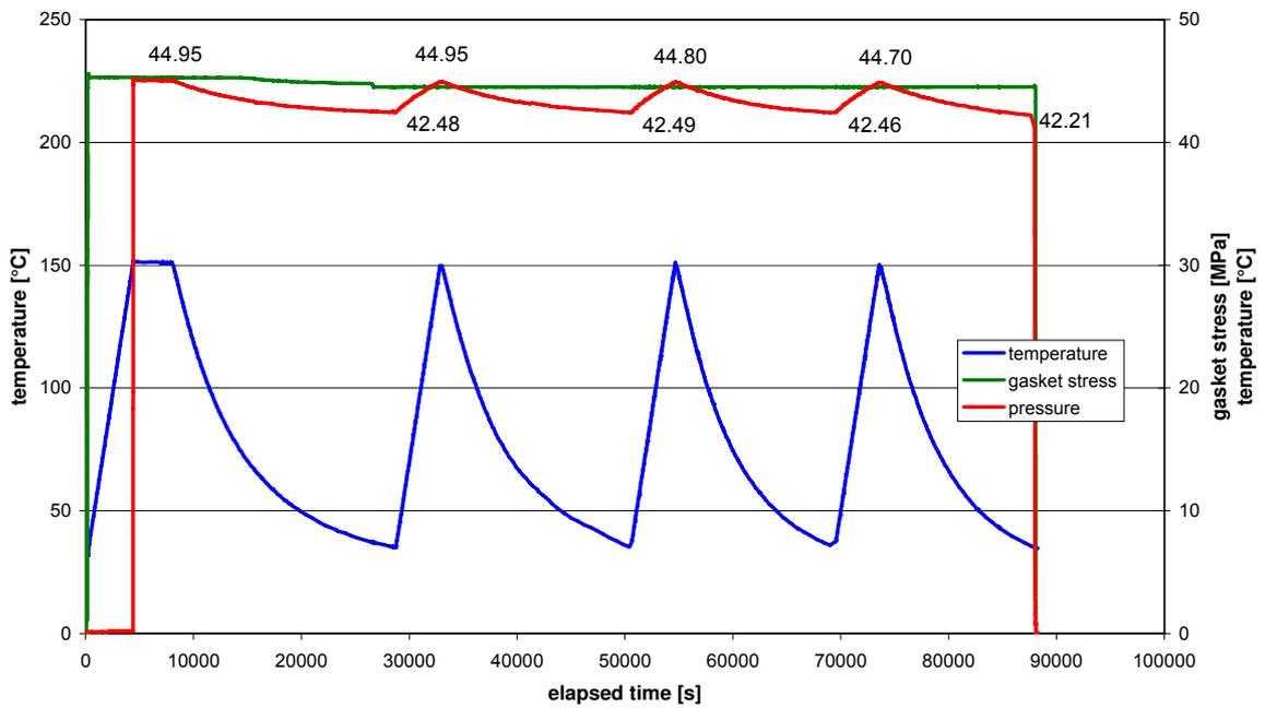
**Shell cycle test at 150 °C according T-2.232686**
