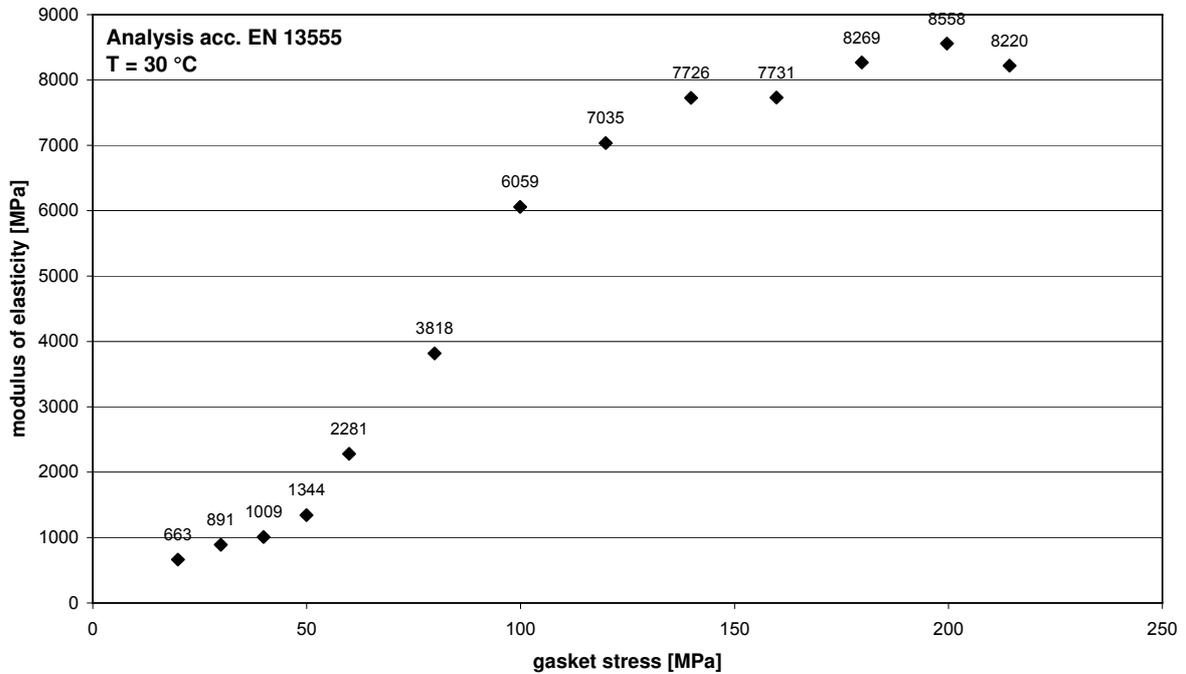
**Compression test (RT) according EN 13555**
