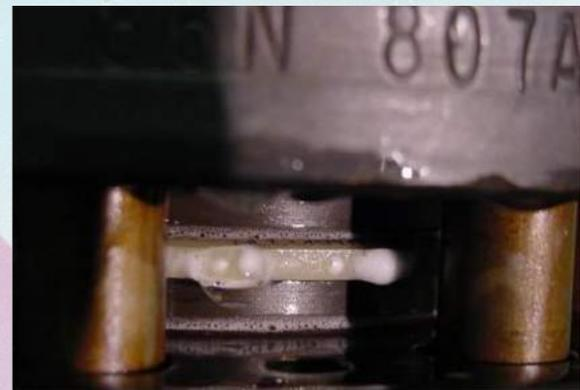
The pressure of the media permeates through the GRE, then contacts the angle in the groove and is forced at an upward angle. The force then pushes the seal against the flange face creating a tighter seal. This works well for surface leakage,
