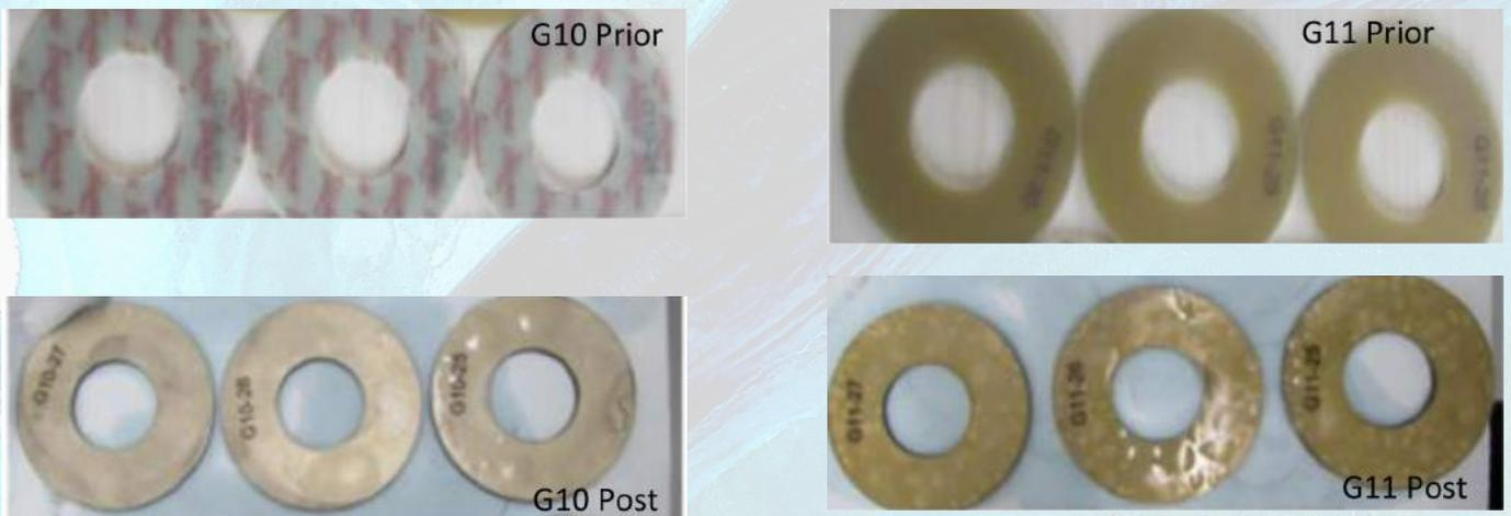
As you can see, both the G10 and G11 had a significant amount of bubbling on the surface of the gasket samples. Density, mass and volume were all tested before and after the test as indicators for chemical attack. Both the G10 and G11 had major shifts in all three areas (see graph below):
