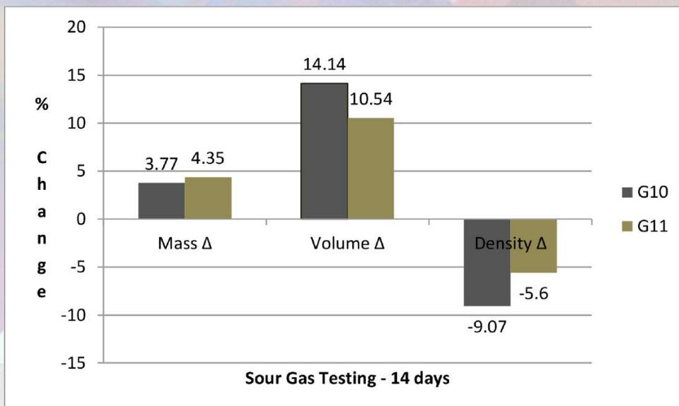
Changes of this magnitude in a 14 day period indicate chemical attack of the material. An isolating gasket that loses density and gains volume is more likely to blow out at high pressures.
