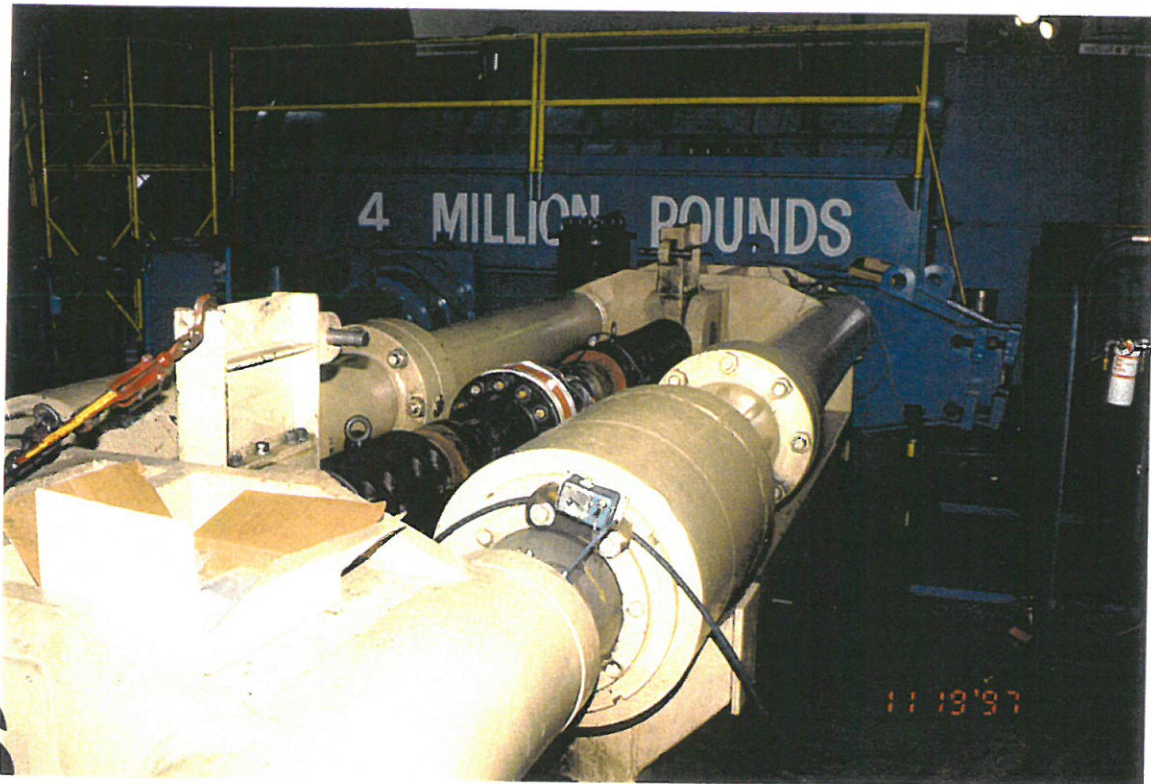
Figure 6 Photograph of the flange assembly installed in the load frame
